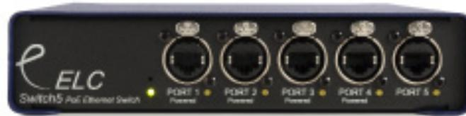
The switch5 is a 5-port Truss-mount Ethernet switch for professional use. The sturdy touring case is equipped with an integrated M10 thread and a locking eye for quick and secure truss mounting. Five LEDs provide information about link and data presence. The dmXLAN switch5 offers four 10 / 100BaseT Neutrik Ethercon ports and a 10 / 100BaseT Neutrik Ethercon Up Link port.
