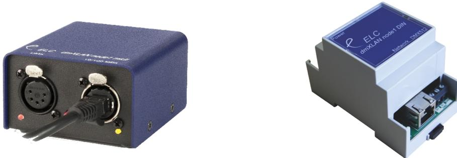
The node1 mkII is a surface mountable DMX / network node with DMX (input or output via 5-pin XLR) and network connection (Ethercon). Power is also supplied via the unit's Ethernet connection via PoE (Power over Ethernet). Programming is completed via the free ELC dmXLAN software.
