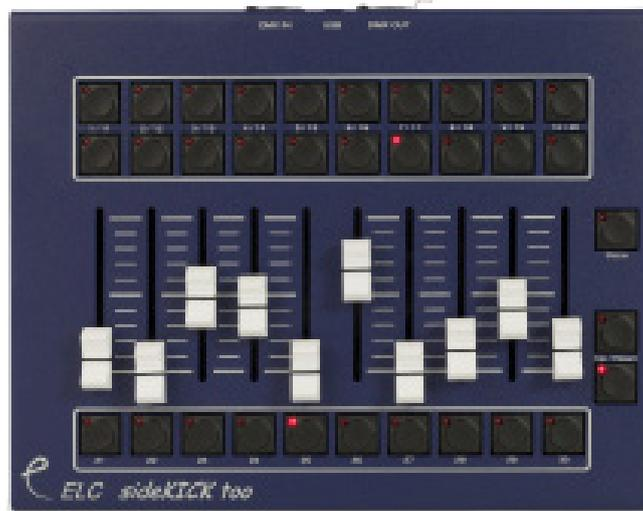
The sideKICK too provides a simple to use DMX scene capture and playback of 30 memories, each of which can be a single lighting state (up to 512 channels) or a chaser with individual period and crossfade times.
