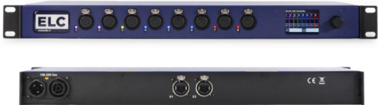
The dmXLAN node8GBx DMX / Ethernet Node comes with an integrated dual GBit ports and colour touch-sensitive display. It offers 8 bidirectional 5-pin XLR female connectors (optically isolated) on the front panel, which can be used as DMX outputs, DMX inputs or DMX outputs with RDM. The two Gigabit Ethercon ports are located on the rear of the unit.
