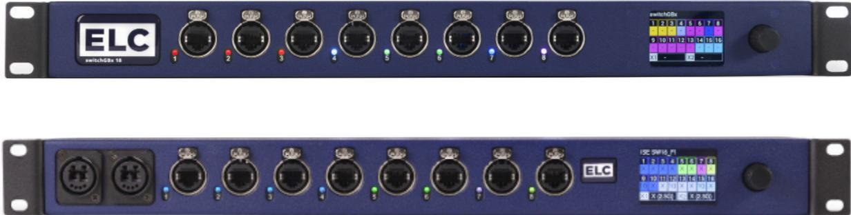
The dmXLAN switch GBx 18 is a programmable 1 gigabit switch (10/100/1000). It has been designed specifically to meet the needs of events to reliably handle the high volumes of data used in light (e.g. Art-Net), sound (e.g. DANTE), and video protocols.
