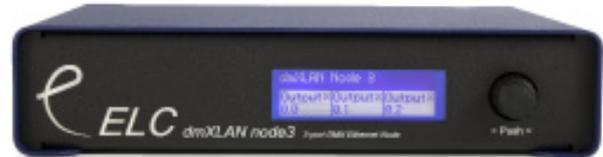
The node3 is a DMX / network node with three DMX (input or output via 5-pin XLR) and two network ports. Programming is easily achieved with the help of the free dmXLAN software or via the LCD display. There are five versions to choose from.
